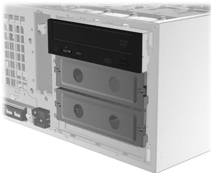
Figure 3-9 Reinstalling the optical drive
